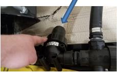
Clean any debris from filter and housing. Then reinstall.
