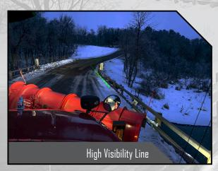
HIGH VISIBILITY LINE allows you to keep your eyes on the road and in control of the vehicle. The WINGLINE™ instantly projects a line in front of the vehicle directing the operator where the trailing edge of the wing plow will be, seconds before it arrives. This not only reduces liability, but also reduces operator fatigue and neck strain.
