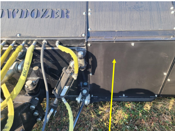
Solid 8' back—no channel for wing cylinders (OLD)
