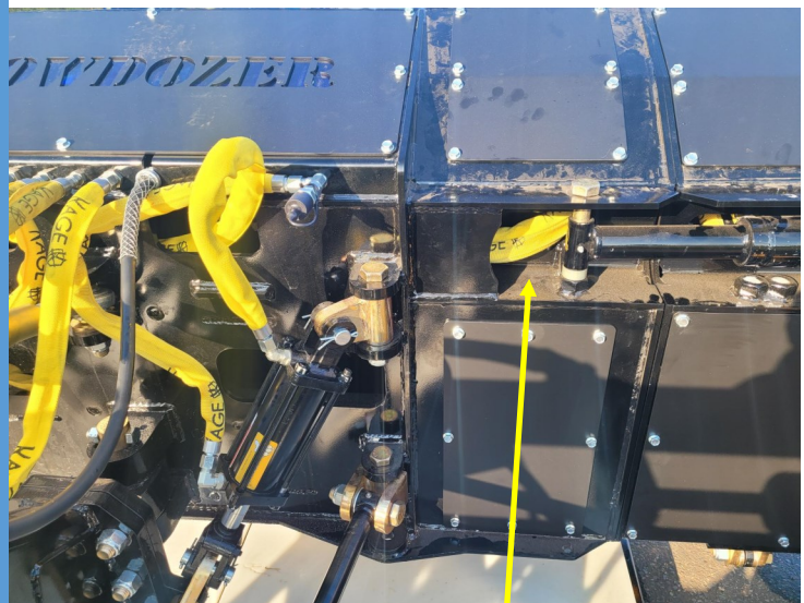
Opening in 6' back for wing cylinders (NEW)
