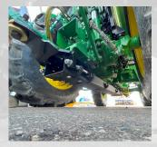
Ground Clearance All KAGE Under-Hitch options are designed to provide maximum ground clearance at the center of the tractor
