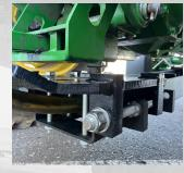
Drawbar Slide The threaded adjustment rod allows keeps the frame tight to prevent slop and egging out of bolt holes.
