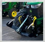
Front 3-Pt Hitch Front 3-point can pick up CAT II attachments and the top link easily stores with an easily accessed pin.
