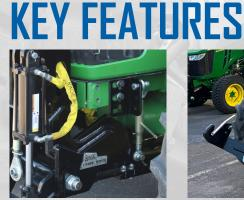
**4-Point Installation** Install the Under-Hitch to virtually any tractor in 2-3 hours, bolting it to the bumper, drawbar & 2 stabilizers.
