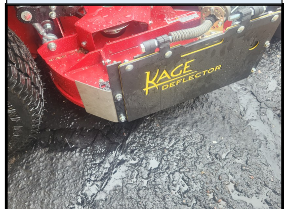
Fig. 5 Block-off plate on a Grass Deflector
