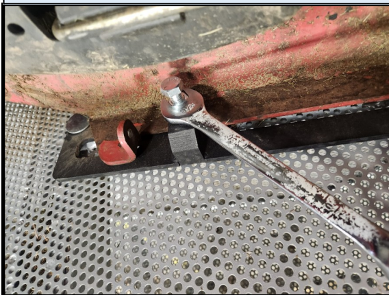
Fig. 3 Tightening bolt on an Exmark manifold
