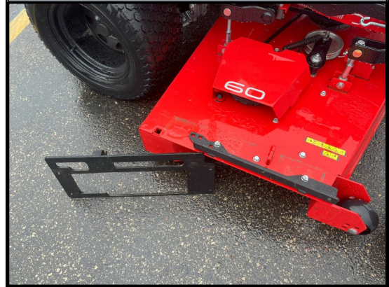
Fig. 1 Bracket installed on a Gravely
